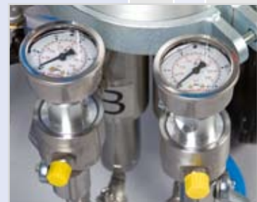
Pressure gauge units at machine outlet for component A and component B
